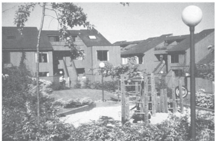
Fig. 21. A human-scaled setting is created when the ratio of the height of the buildings to the width of the shared outdoor space is carefully considered (Housing Co-op, Vancouver, Canada).
